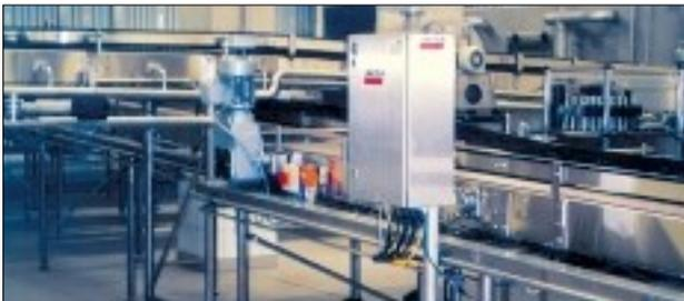
Section of a filling line with ejector cabinet
