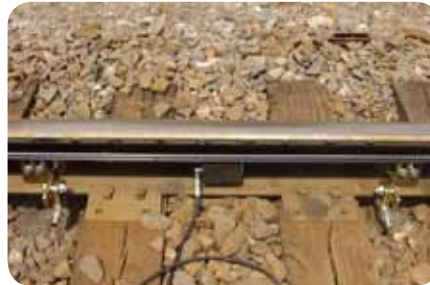
Lincoln's wiper bar – open, clean ports
