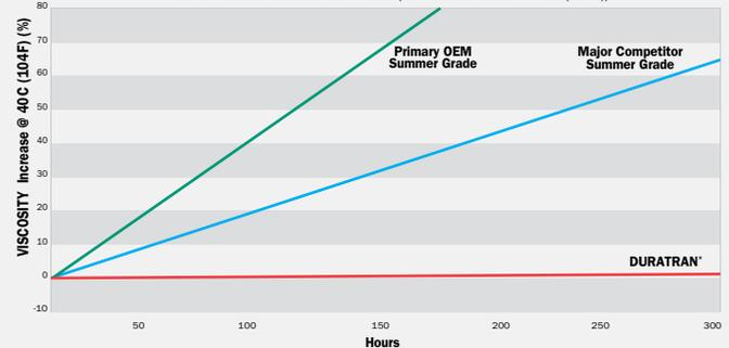
\*Note: Results are after 300 Hr ABOT Oxidation Test which is more severe than JD requirement Allison C-4 (GM 6137M) Oxidation Test.
